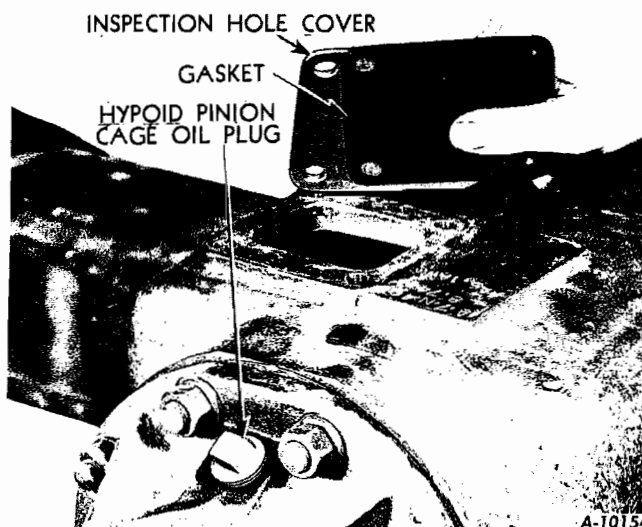
Fig. 8 - Insert one pint of lubricant in pinion cage before starting new truck or after overhaul.
